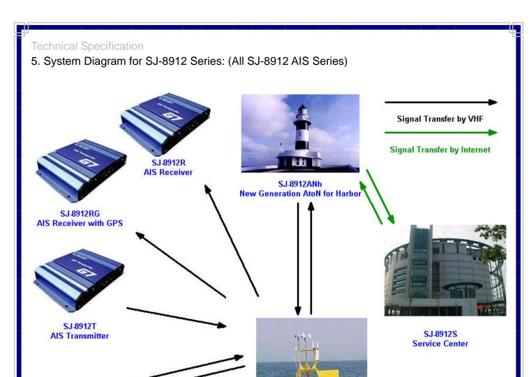
User can have multiple SJ-8912ANo and SJ-8912ANh connected together to monitor all your vessels around the world with just one SJ-8912S Service Center.
